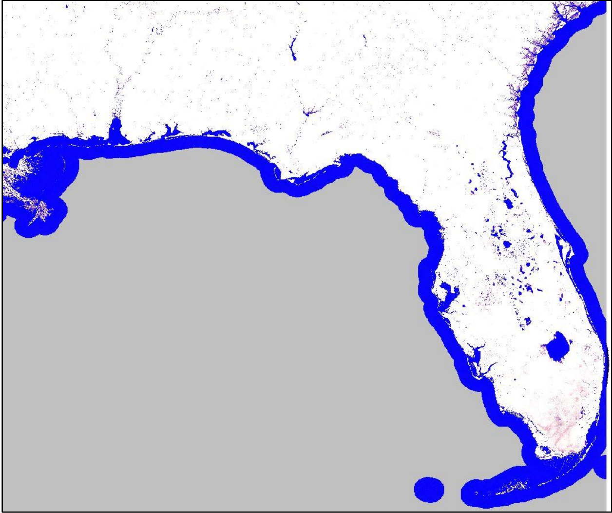
Figure 8 Water mask for eliminating subtidal and perennial water areas from Landsat imagery after Pekel et al. (2016).
