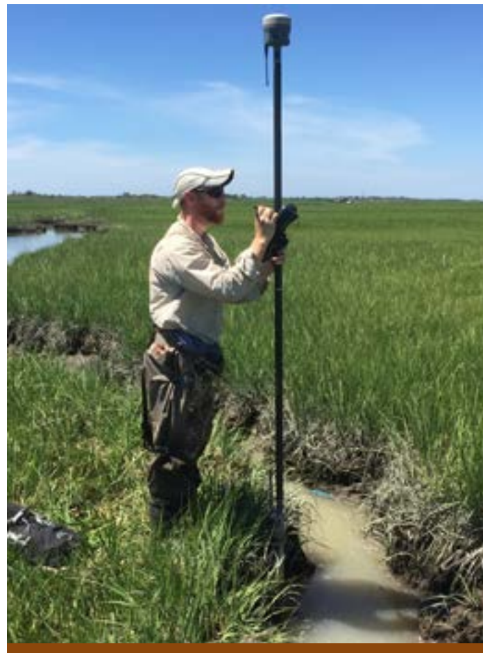
Andrew Neil, a cooper at the University of Rhode Island, collects elevation along a ditch at Fire Island National Seashore. Points were established using a 20-m grid which covers the range of elevation and vegetation types in the salt marsh. NPS
