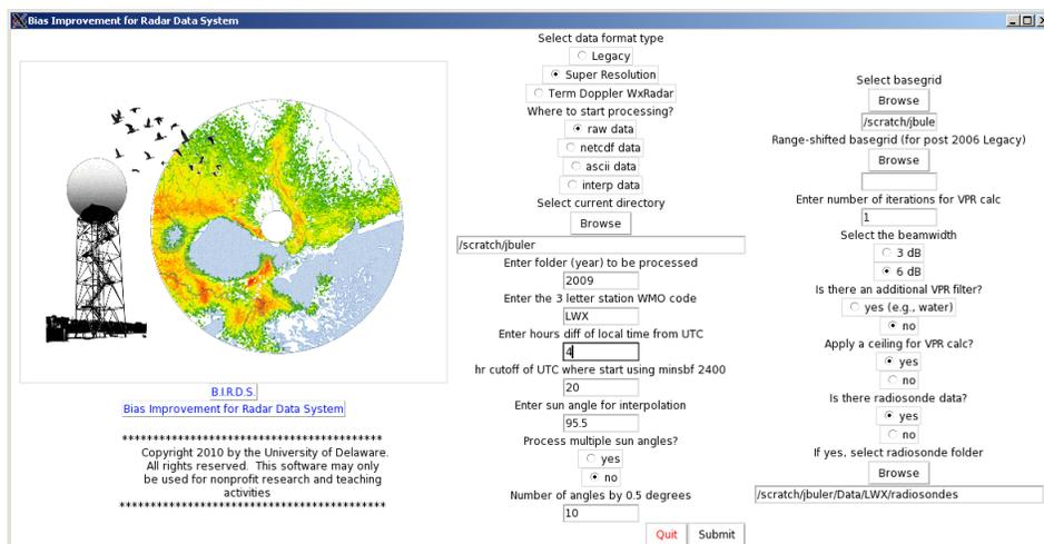
Figure 4. Graphical user interface for the BIRDS software developed at the University of Delaware. BIRDS processes raw radar data from multiple dates at one radar, and summarizes bias-adjusted reflectivity measures from every sample volume in the radar-sampled area.
