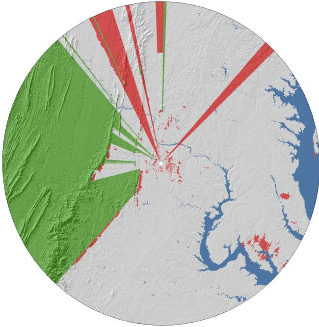
Figure 3. Masking map of the LWX radar in Sterling, VA, showing sample volumes excluded from analyses due to 1) topographic beam blockage (green), 2) dominance of open water (blue), or 3) persistent ground clutter contamination and other sources of beam blockage (red) .
