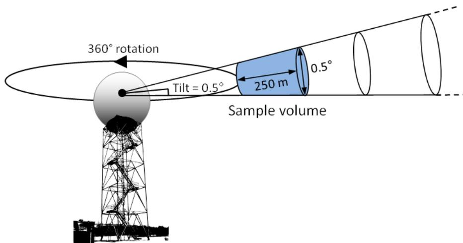
Figure 2. Illustration of operation and individual sample volume of a WSR-88D. Not drawn to scale.
